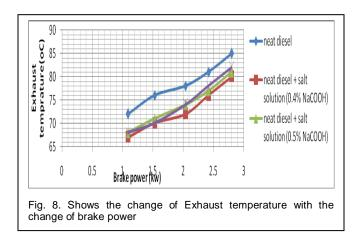
It is seen that the temperature is gradually increased with brake power. But it is comparatively lower than neat diesel by using salt diesel emulsion because water diesel emulsion reduces the temperature of the combustion region.
