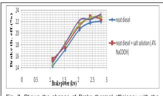
Fig. 7. Shows the change of Brake thermal efficiency with the change of brake power
