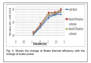
It is seen that the brake thermal efficiency is increased as the BSFC is reduced significantly for using salt diesel emulsion.
