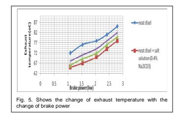
It is seen that the temperature is gradually increased with brake power. But it is comparatively lower than neat diesel by using salt diesel emulsion because water diesel emulsion reduces the temperature of the combustion region.
